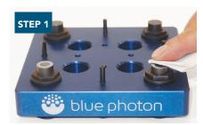
Clean dirt and oil from the grippers and workpiece.
