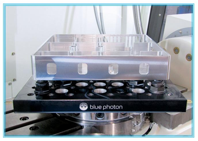
**ADHESIVE WORKHOLDING** the universal part gripping solution
